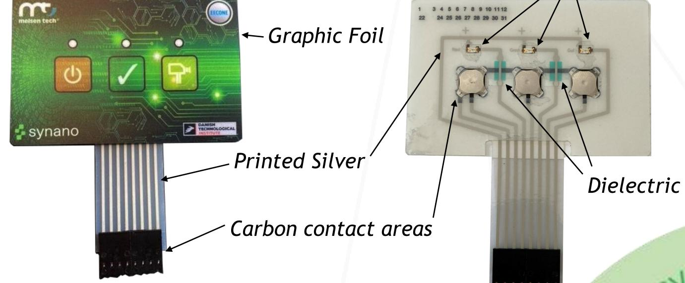
Membrane switch/keyboard consists of a PE circuit using screen-printed silver, dielectric, and carbon materials on a poly(ethylene terephthalate) (PET) foil. Light emitting diodes (LEDs) are mounted on top, and the entire foil is laminated with several plastic layers, including the front graphic foil. Screen printing is the standard method used for membrane switch production.
